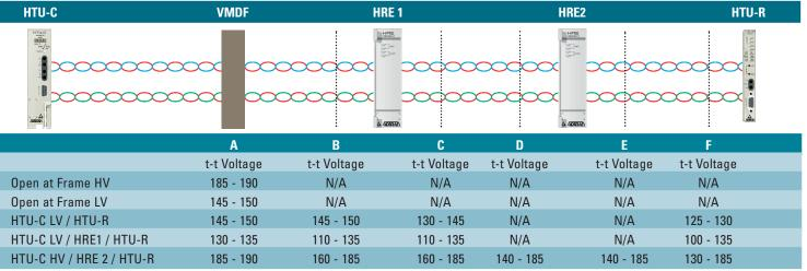
**NOTE:** All measurements taken with HTU-C installed. With the HTU-C unseated or with protector removed at VMDF, t-r resistance will be cable resistance plus 3 ohms (for either HRE or HTU-R).
